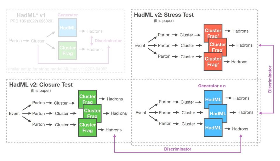
Protocol for fitting a deep generative hadronization model in a realistic data setting, where we only have access to a set of hadrons in data.
